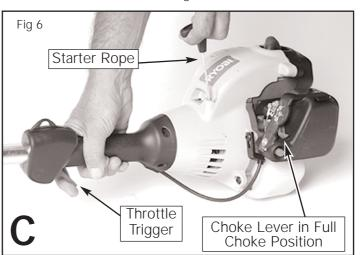
Place the CHOKE POSITIONS Fia 7 choke lever in the "Partial Choke" position. Fig 7. Keep the throttle trigdepressed at all times. Pul the starter rope briskly 1 to 3 times
